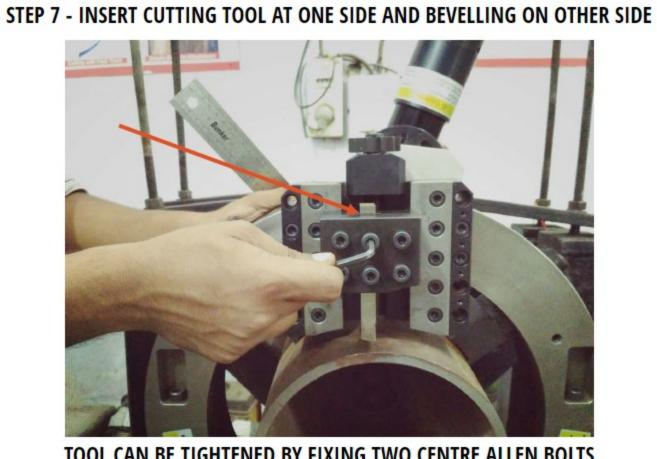
TOOL CAN BE TIGHTENED BY FIXING TWO CENTRE ALLEN BOLTS
